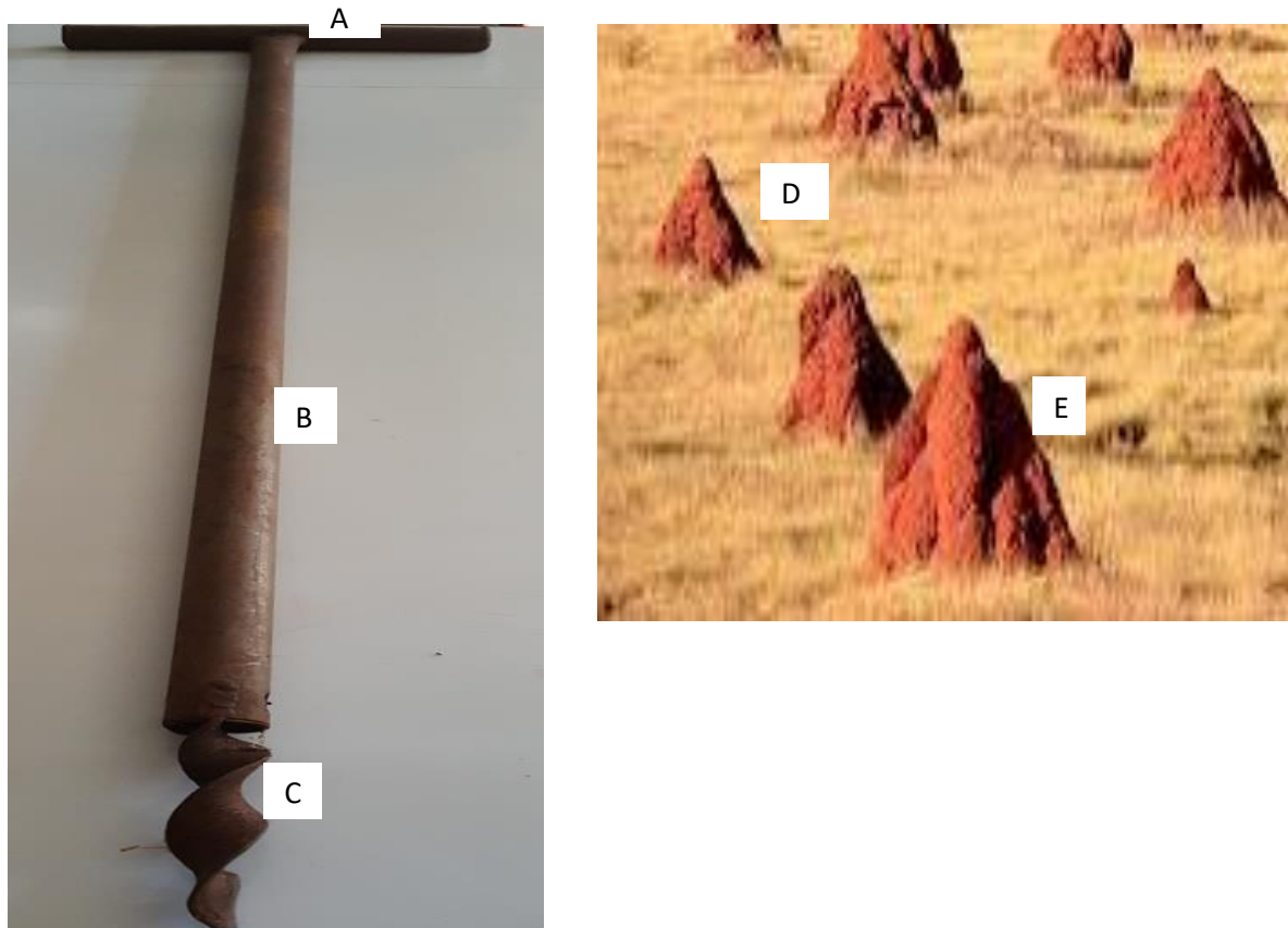
Figure 8: Termite mound injector (A) top handle (B) injection hole (C) curved mound cutting edge (D) small size mound and (E) medium to large mound size.
