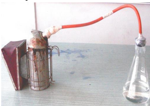
Fig. 1. Setup of the beekeeper's smoker for the preparation of plant-derived aqueous smoke extracts.
