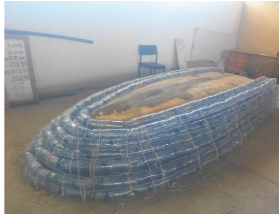
Fig 7c) The bottles are tied together by weaving together alternative rows so as the ropes should not fall apart.
