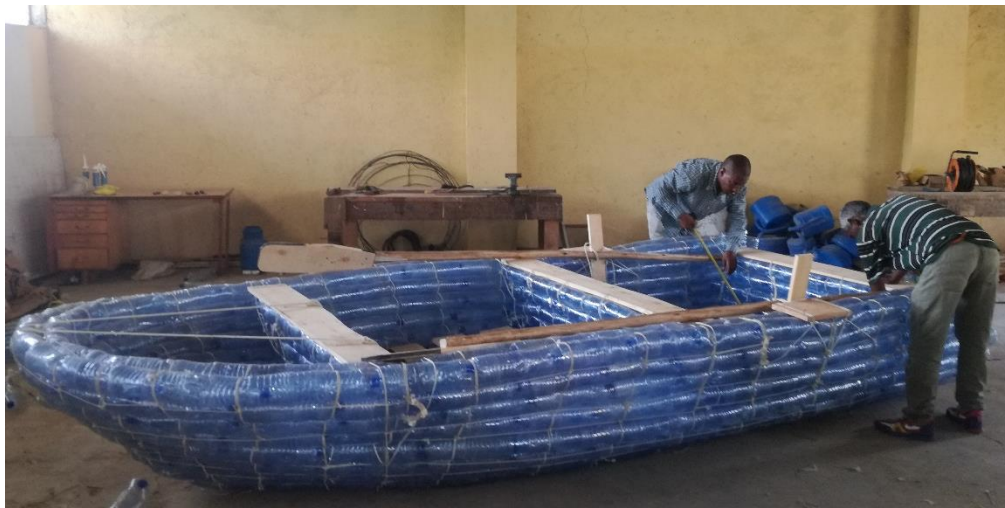
Fig 7e) tying plank for the sitting area
