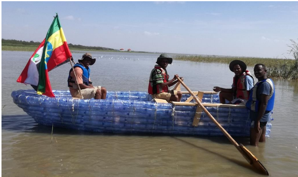
On lake evaluation of boat constructed from plastic bottles
