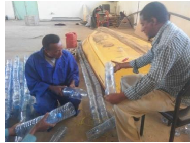
7b) cutting and making the bottles in row
