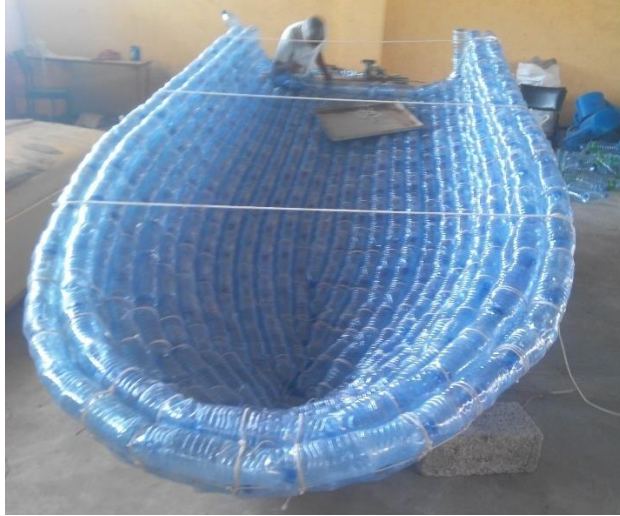
Fig. 7d) reinforcing the sides with rope
