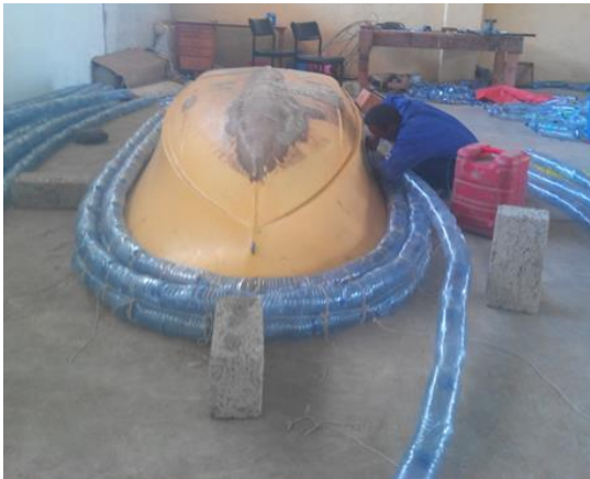
Fig 7c) The bottles are tied together by weaving together alternative rows so as the ropes should not fall apart.
